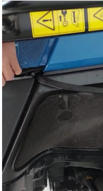
Figure 14: Hood of the tractor is loose
