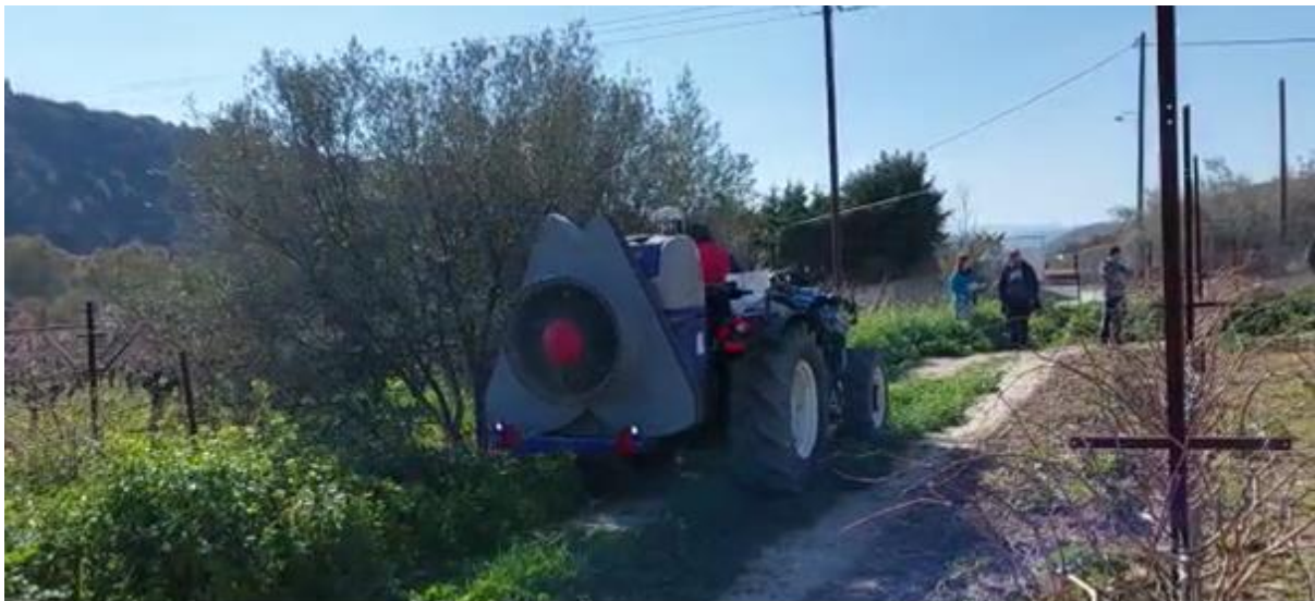
Figure 10: Perception unit, AGC box and sprayer worked well on olive trees
