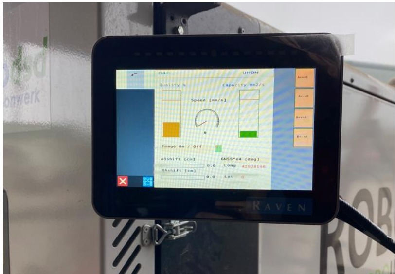
Figure 19: VT mounted on the Robotti showing live values of speed and weeding quality
