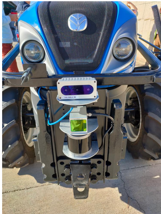
Figure 8: Sensors for navigation unit mounted on R4C tractor
