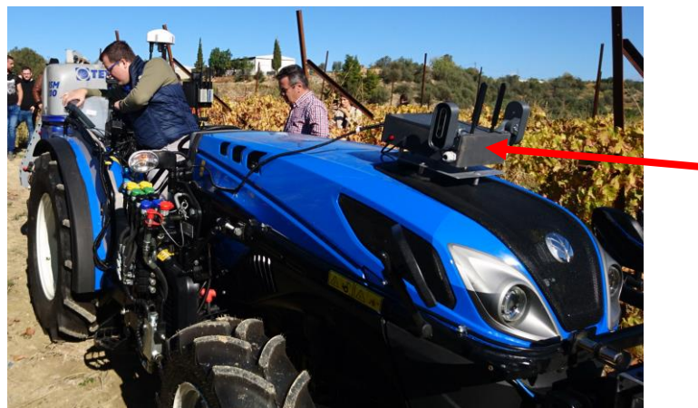
Figure 7: Crop perception unit mounted on R4C tractor
