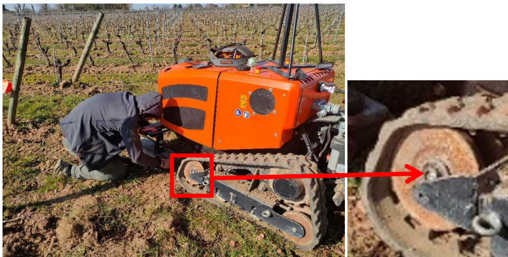
Figure 5: Broken front roller of one of the tracks of the CEOL robot
