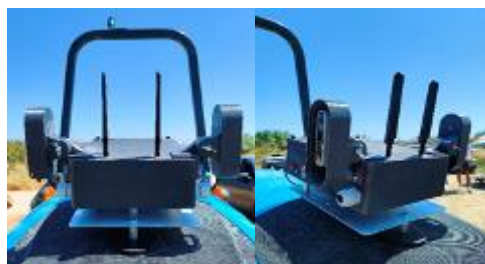
Figure 13. Perception Unit system mounted in the front part of the tractor during field trials.
