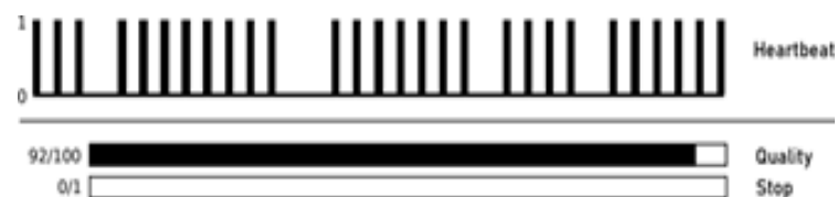
Figure 4. Irregular sensor heartbeat, quality is impacted slightly but stop is never triggered.
