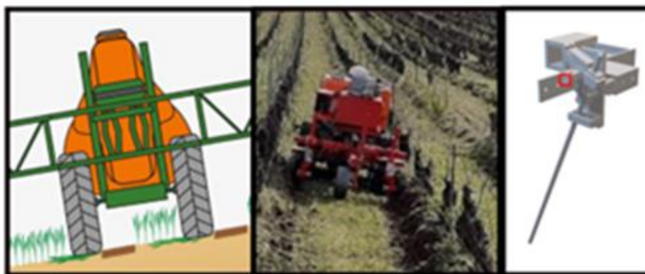
Figure 2. Depth check tool: a) An illustration of how slope shifts the wheels. b) CEOL robot shifted due to the slope and the cutter won't work in one side. c) A custom build tool to detect the distance and in the red square is the rotary encoder.
